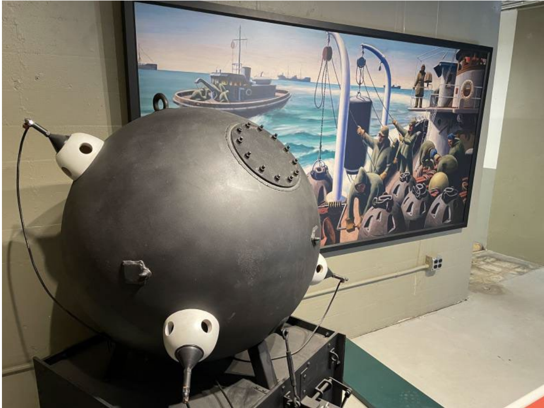
The Fort Miles mines were connected to a central command center. A passing ship would trigger a signal to Mine Command personnel.
